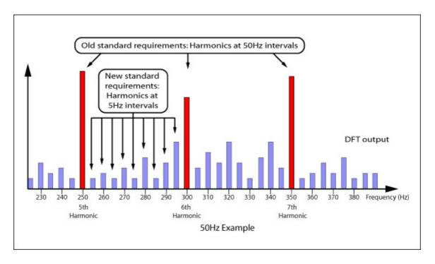
The PM6000's use of discrete fourier transforms (DFT) as opposed to the conventional fast fourier transform (FTT) means that it can achieve the required accuracy with ease. In this way, the Voltech PM6000 power analyser provides design
